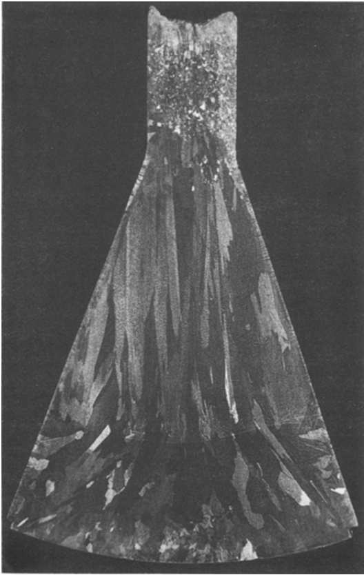
Figure 5 Macrostructure of a lead ingot showing the curvature of the solid/liquid interface due to a sudden change of solidification rate.
